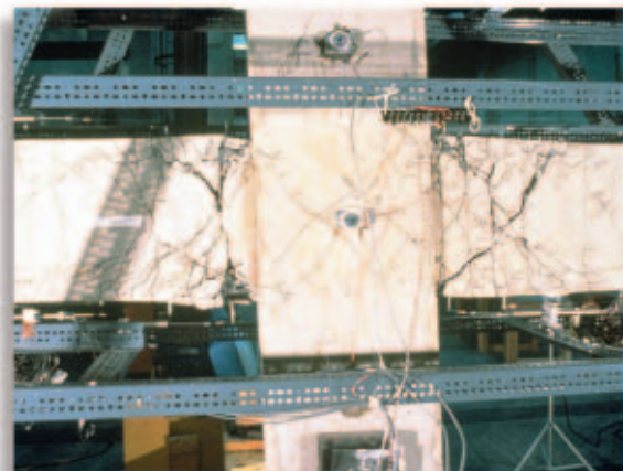
Crack pattern of cast-in-place frame assembly at 3.5% story drift.
