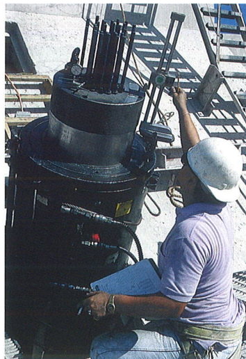
measurement of piston stroke
